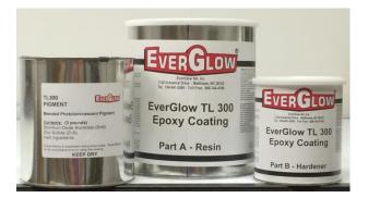
TL300 is a high build, high luminance epoxy coating that is designed to be thoroughly mixed at the work site and applied within 30 minutes onto a horizontal surface. The desired dry coating thickness should be 25 - 35 mils thick for uniform coverage. It should be applied over a white primer which is appropriate for the installation surface and compatible with the TL300 coating.
