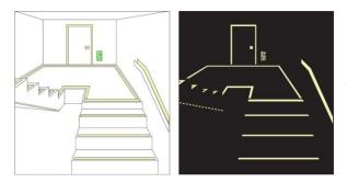
EverGlow tapes used to mark handrail, landing perimeter, exit door framed and door hardware.
