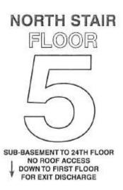
FIGURE A.7.2.2.5.4 Example of a Stairway Marking Sign.
